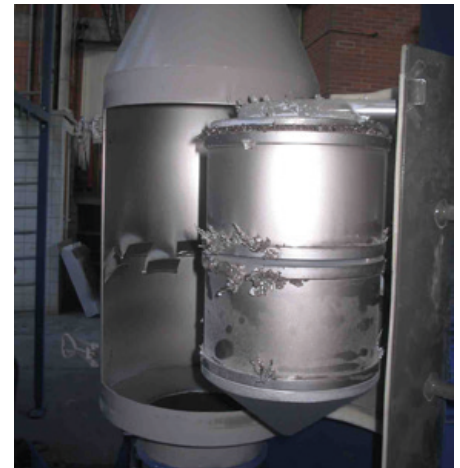
An upside down mounted bullet magnet for plastic granulate
