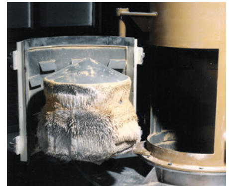
Bullet magnet for ceramic material
