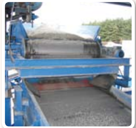
A Neoflux® Drum magnet , for catching Ferrous parts of 0-10 mm in a glass recycling process.
