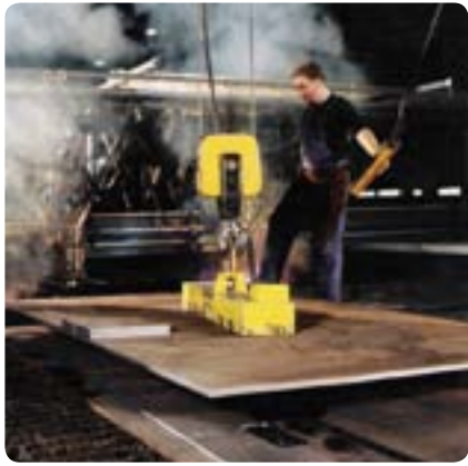
Electro lifting magnet for steel plates.
