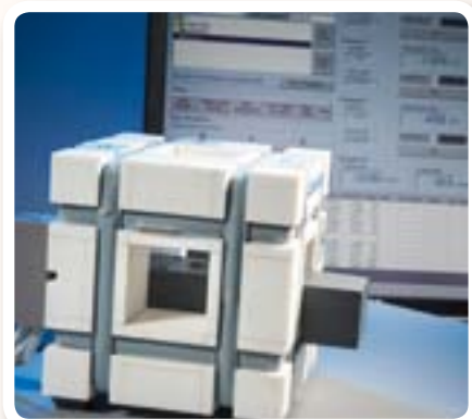
Goudsmit Supplies has a 3D Helmholtz coil, that can be used to measure the magnetization angle.
