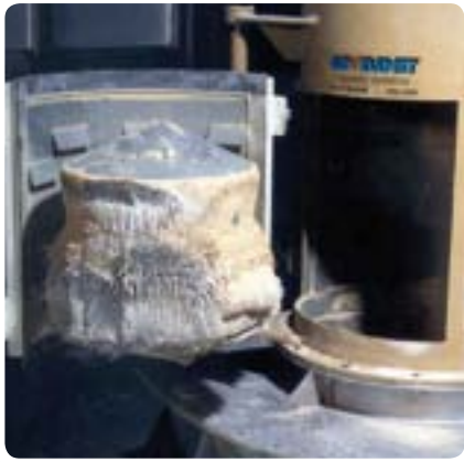
A pipe magnet removes iron particles from various powders and bulk goods, among others, from fire-brick (ceramic industry).
