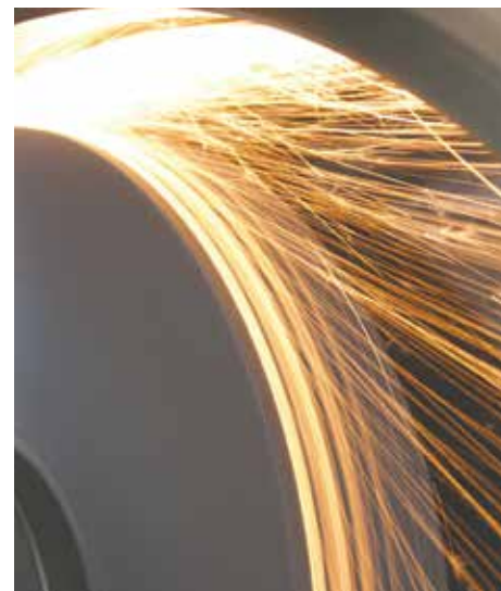
Grinding die surface ▲
