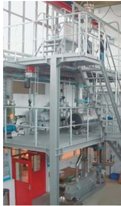
SCHULE pilot plant with continuous cooking plant for grain, parboiling, food, bulgur, etc.
