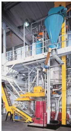
KAHL pilot plant: Proportioning unit, continuous mixer, hydrothermal reactor, annular gap expander, extruder OEE, flat die pelleting press, belt drier/cooler, Rotospray, crumbler, crushing roller mill
