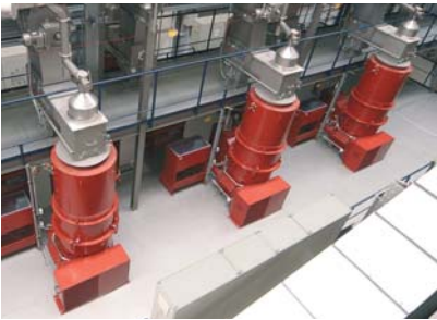
Domestic-waste pelleting plant for the production of pellets or fluff
