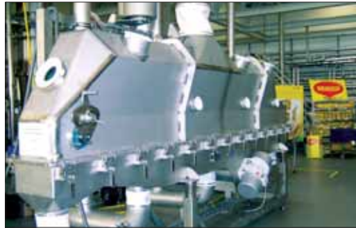
Figure 23: Vibrating fluid bed dryer VF 40/3,5 in a development center
