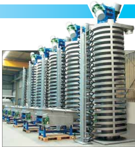
Figure 26: Cooling spiral conveyors 1400 mm diameter width, with upstream screening machines for screening and cooling 3000 kg/h plastics granules each
