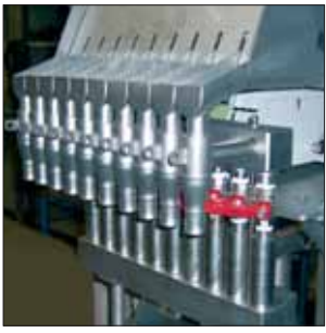
Figure 11: ER batching conveyors in special design for proportioning of catalysator granules
