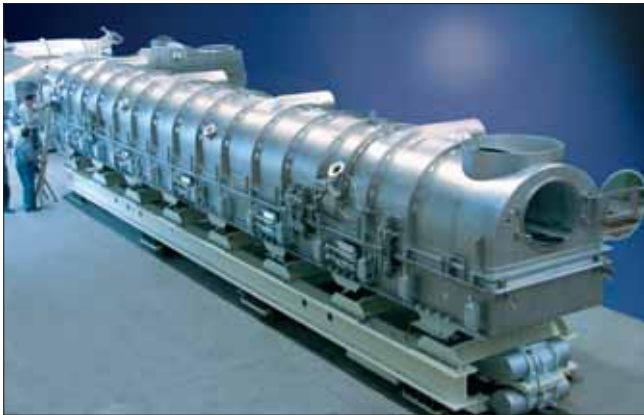
Figure 24: Natural frequency fluid bed dryer/cooler 22 m 2 area
