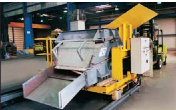
Figure 15: Charging conveyor for furnace feeding
