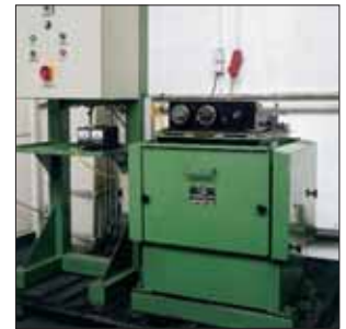
Figure 20: Vibrating table for mechanical strength testing
