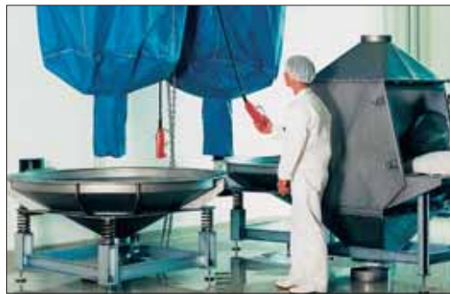
Figure 17: Vibratory equipment for discharging of big-bags and bags
