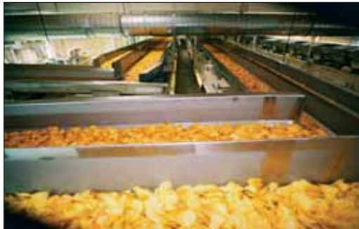
Figure 3: Partial view of a vibrating conveyor plant with an overall length of 120 m used to convey potato chips at a rate of 60 m 3 /W.
