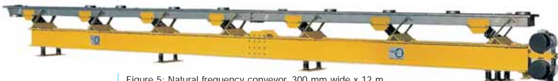
Figure 5: Natural frequency conveyor, 300 mm wide x 12 m long, handling 10 t of detergent an hour
