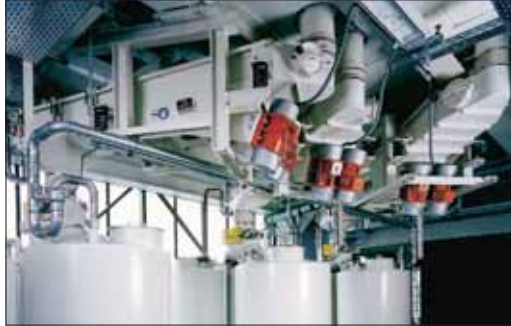
Figure 2: Vibrating trough conveyors in a chemical plant
