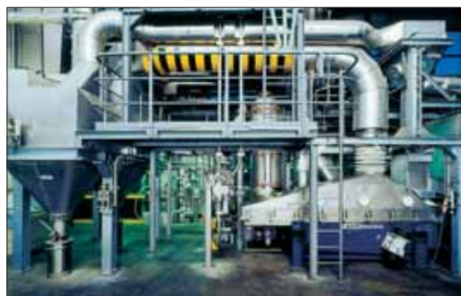
Figure 24: Natural frequency fluid bed dryer/cooler 22 m 2 area
