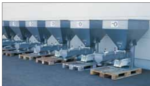
Figure 19: ER vibrating feeders with hoppers
