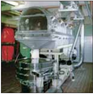
Figure 21: VF 40/10 vibrating fluid bed dryer in a food processing factory
