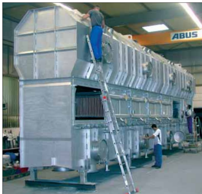
Figure 28: Fluid-bed dryer, fluid-bed area 26 m 2 , with integrated slide-in steam coils for a detergent intermediate product
