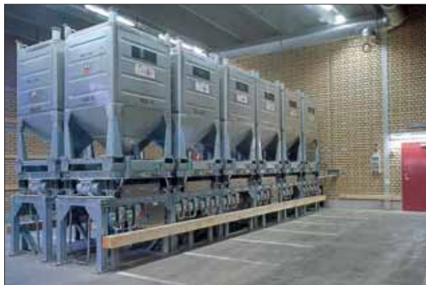
Figure 18: Vibratory frames for discharging of containers
