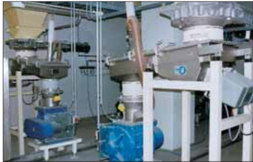
Figure 13: Bin discharging trough conveyors with electromagnetic vibrators
